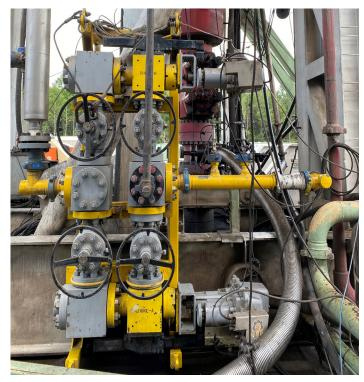
Our fit-for-purpose MPD hardware is integrated with rig structure for maximum flexibility.
